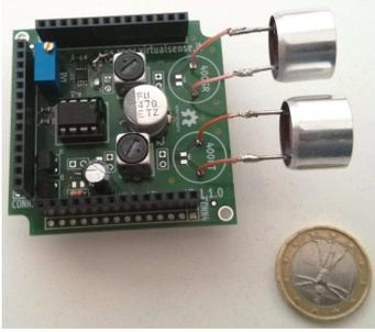
**Figure 1: Prototype of the ultrasonic wake-up module.**
